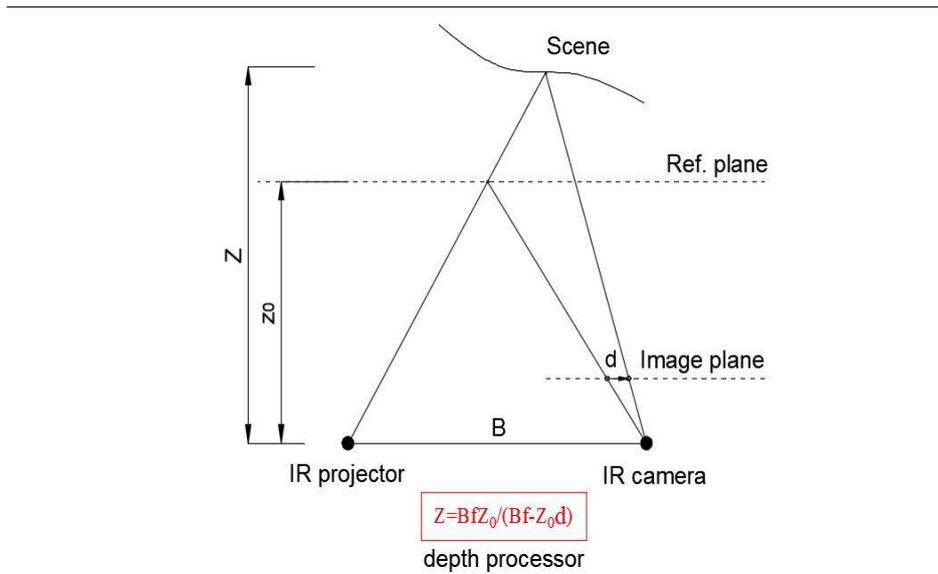
FIG 1 SCHEMATIC DIAGRAM OF THE MONOCULAR STRUCTURAL OPTICAL IMAGING PRINCIPLE
